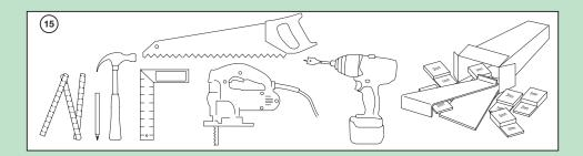
When cutting the Pergo plank, be sure you are not creating splinters or chipping when cutting. If using a hand saw, keep the decorative surface faced up, and if using a jigsaw keep the decorative surface
