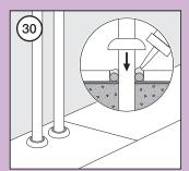
To secure extra water protection around the perimeter of the floor and avoid water to enter underneath the panels, apply the flexible PG Aqua Sealant up to the wall base, thresholds, door frames, pipe covers etc.
