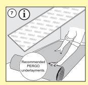
Pergo laminate flooring must not be installed in a typical wet room or in rooms with a floor drain.
