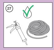
Sealing the perimeter expansion joints combines the compressible PE foamstrip (NEFOAMSTRIP) with diameter 8 to 10 mm and the flexible and waterproof PG Aqua Sealant. Push the PE foam in the expansion joints and apply the transparent PG Aqua Sealant under slight angle towards the Pergo - Sensation floor. Install the wallbases with PG Multiglue (PGGLUE290). Apply the flexible PG Aqua Sealant between wallbases and floor to avoid
